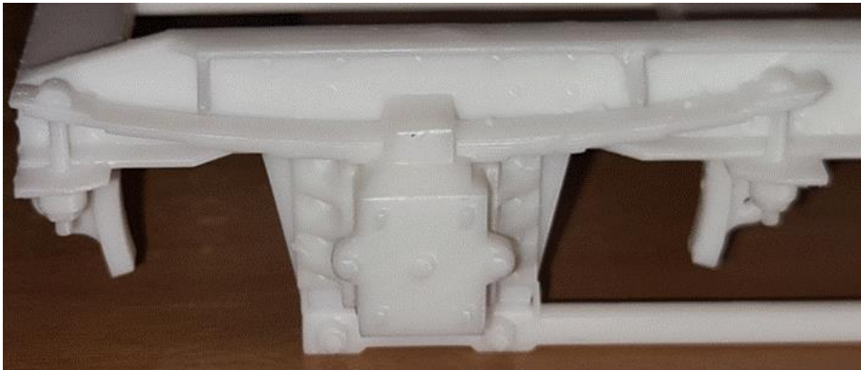
The level of detail possible with resin printing.
