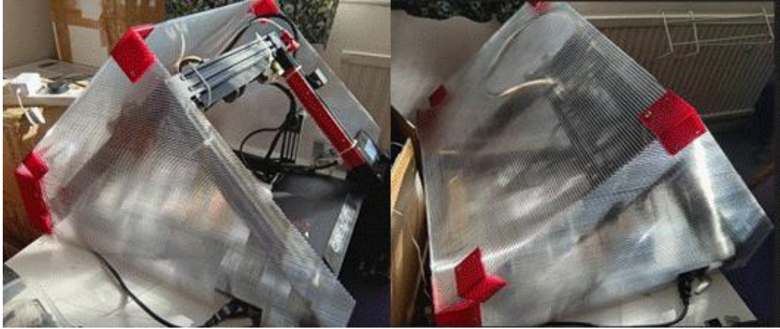
Illustrating the 3-D printed corner bracket fixings (visible in red)
