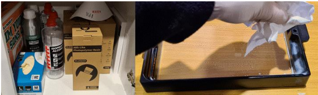
Storage of materials including gloves, filters, IPA and resin in a dark cupboard (to the side of the computer desk where it is easily to hand). On the right, cleaning the resin tray. Note the clear FEP at the base to let the UV light through.
