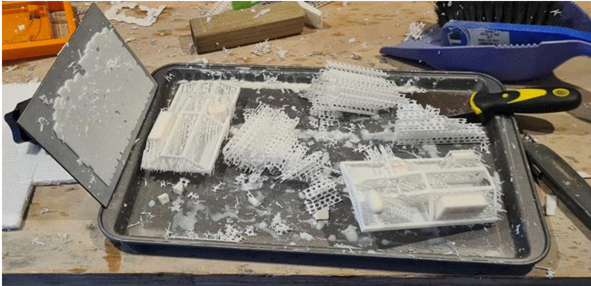
The oven tray and build plate et al on the workshop bench with two prints cut away from the scaffold. The platform is still stuck on the build plate.
