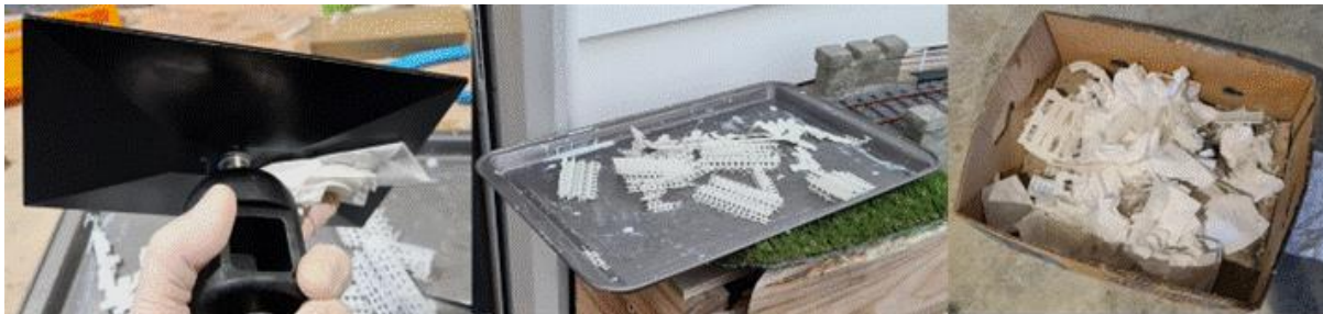
Left: cleaning the build plate in the workshop: note the gloves. Centre, the discarded debris being cured outside and; right, finally discarded in the dedicated cardboard box for disposal with the general rubbish.
