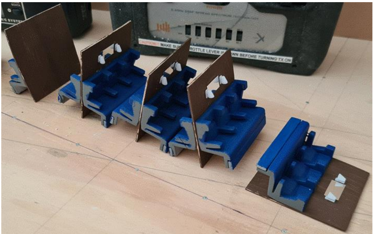
An example of the use of different systems used to make up components for the main models. These are first-class compartment sub-assemblies with 3-D printed seats and lamps, and 2-D cut 1mm birch ply compartment panels with mirrors (from some plastic mirror sheet found at a local craft shop). N.B. whilst the mirror shape was a straightforward rectangle, there were over 40 of these, so cutting them out electronically saved a lot of time and they were far more accurate than could have been managed by hand.
